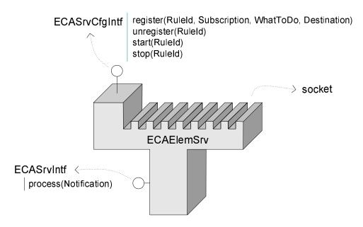
Figure 6.8: Schematic view of the abstract class ECAElemSrv
