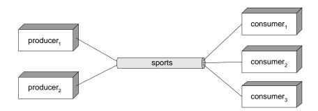
Figure A.2: Channel-based Addressing
