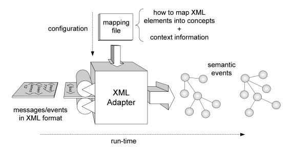
Figure 6.15: XML adapter
